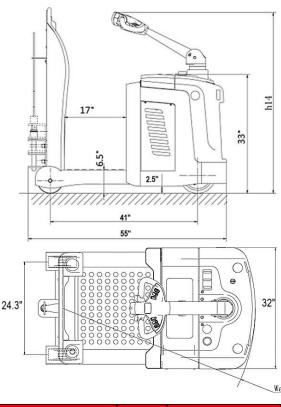
The EKKO EG30 Tow Tractor is designed for tugging and pulling applications made with quality materials, components and workmanship. Every product is robotically welded, powder coated and is reliable for loading and unloading trucks, loading docks, stock rooms, manufacturing floors and warehousing.
