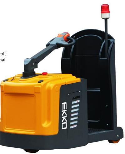
**BRAKES:** Electro-magnetic braking for secure stopping power; Electronic neutral braking for accurate control.
