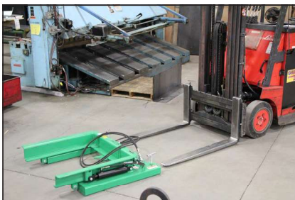
Step 1: Insert forks & secure unit using included safety chain. Connect quick-connect couplers to forklift auxiliary circuit.
