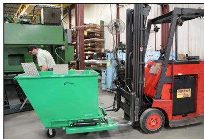
Step 2: Easily roll Mobile Hopper into Forklift Attachment to engage secure latching system.
