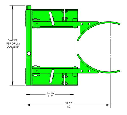
HCG = HORIZONTAL CENTER OF GRAVITY LC = LOAD CENTER LLC = LOST LOAD CENTER VCG = VERTICAL CENTER OF GRAVITY
